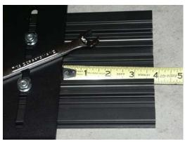
Attach C-B43 transmission hump bracket to 18" section of extrusion using (4) 1/4" x 3/4" bolts and serrated nuts. (7/16" Wrench)
